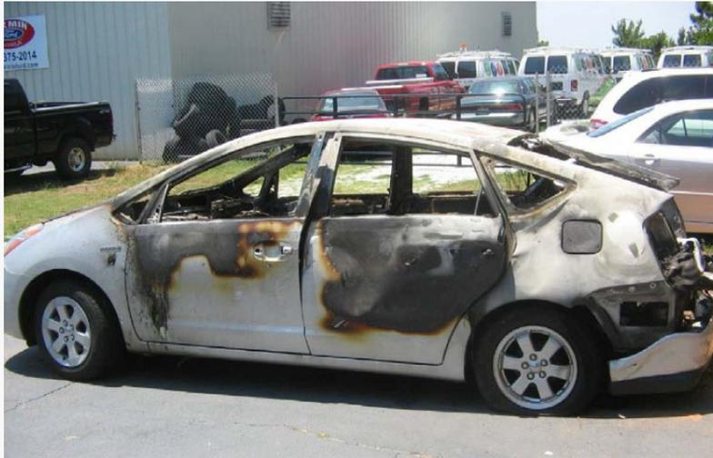
Fire damaged Li-ion cells...
